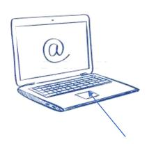
A touch pad (touch panel) is nothing but a touch sensitive surface performing the mouse functions we got to know, which controls the mouse's cursor on the screen by moving our fingers.
